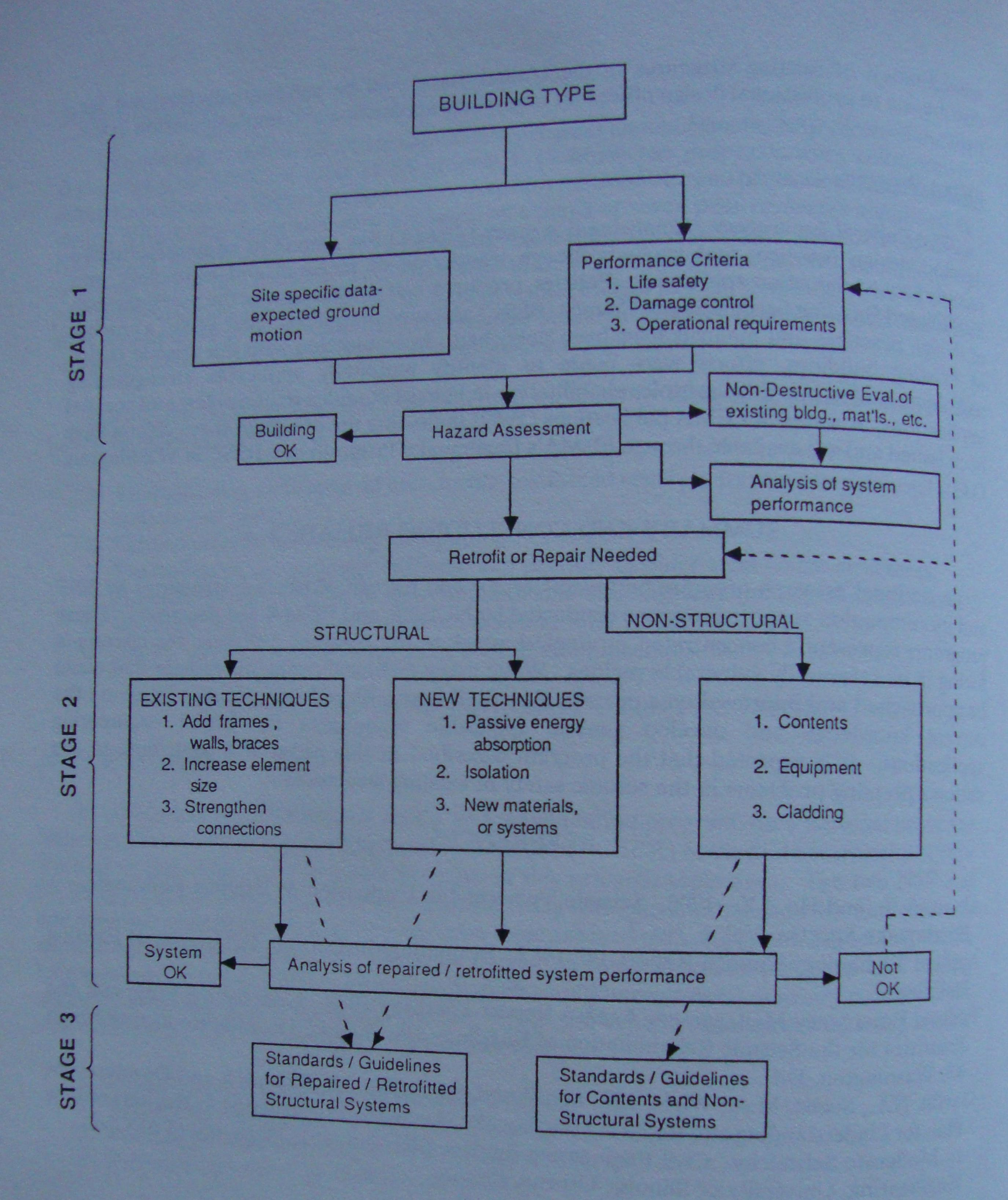
Figure 1. Stages in Hazard Reduction of Existing Buildings (from Los Angeles Workshop)
